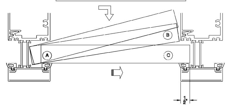
NOTE: The typical glass bite for the I.G. captured system is 1/2", except at I.G. heads, where the glass bite is 3/8". Glass sizes are based on horizontal D.L.O. plus 1" and vertical D.L.O. plus 7/8".
