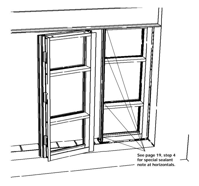
NOTE: On long runs, check overall frame dimensions at every fifth opening to avoid dimensional build-up. The commercial cut length tolerance is +/- 1/16". It is critical to check every fifth unit for location relative to established benchmarks.
