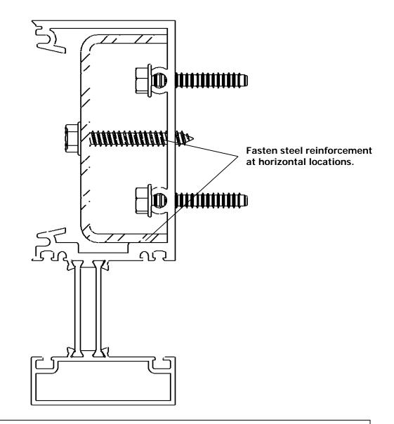
When steel reinforcement is factory installed into the mullions, fasteners will be used to prevent damage or slippage of the steel during shipment. This practice is also recommended for the customer on stock length orders.
