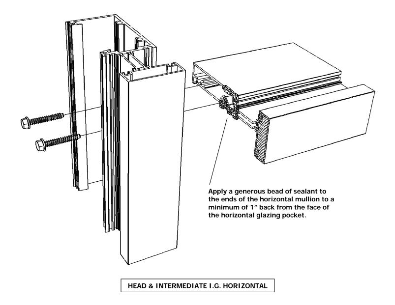
After each frame unit assembly is complete, wipe off all excess sealant, and allow the frame unit to cure.
