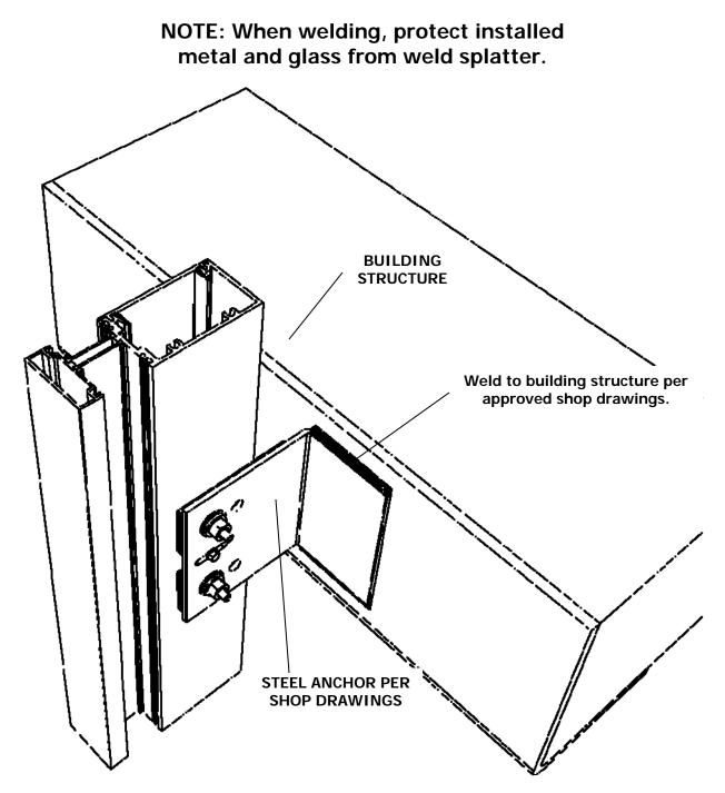
NOTE: The elevation of the structure must be within the adjustment limits of the anchoring system. See approved shop drawings for limitations.
