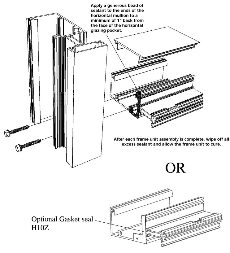
Install gasket to each end of horizontal before attaching to vertical.
