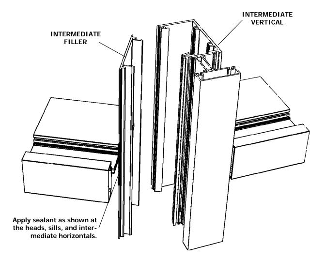
Note: Care should be taken when handling the frames to avoid damaging the edges of the fillers. A block of wood and "C" clamps should be used to aid in snapping the filler to the mullions.
