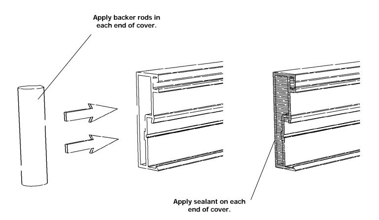
NOTE: Exterior pressure covers to be cut D.L.O. minus 1/8" at typical lites and D.L.O. minus 3/16" for lites on the deep pocket side of the expansion mullions.
